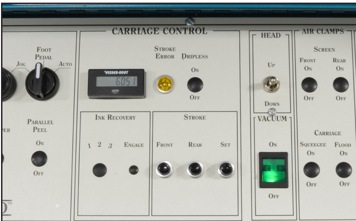
Up-front Stroke Adjustment is computer-controlled through the main control panel or optional touchscreen.
