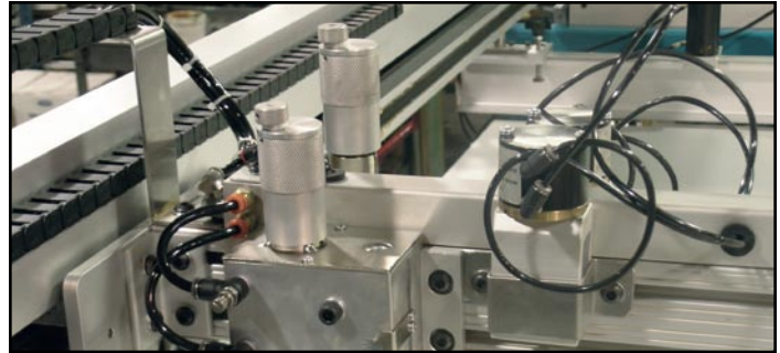
Figure 2. Patented “Squeegeelizer” pneumatic chopper assembly evenly distributes pressure across squeegee blade.
