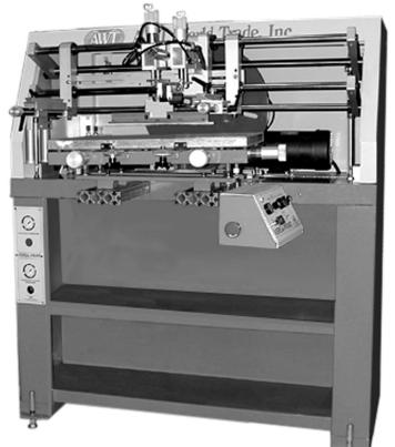
The DI-Versa-Print<sup>TM</sup> uses new technology to print on flat and formed 3D parts as well as on boxes, decals and other industrial objects.
