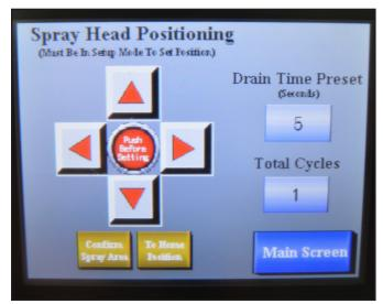
From the convenient control panel, the operator can perform a variety of monitoring and operating functions, including spray head positioning, drain time and total cycles.
