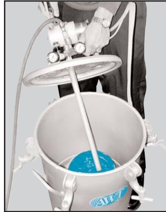
Operator never handles inks or emulsions, which are dispensed through feed tubes.
