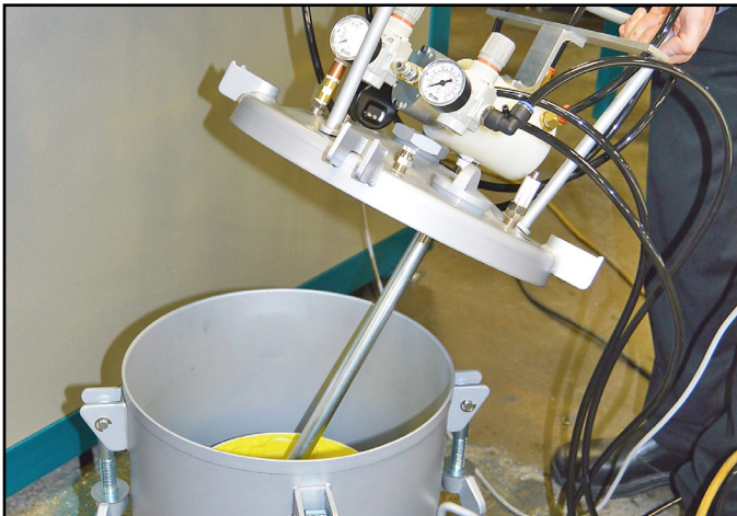
Operator never handles inks or emulsions, which are dispensed through feed tubes.
