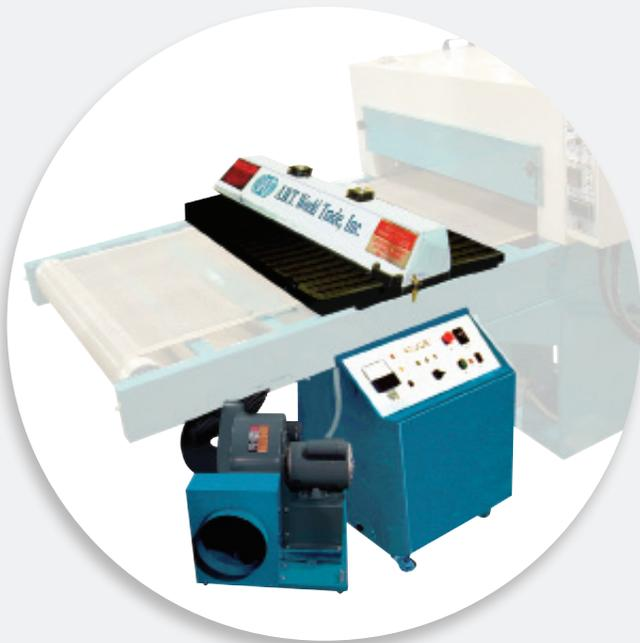
*Existing dryer retrofitted with AWT Curing Head.*
