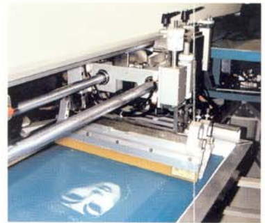
The only independent screen lift system on this style machine
