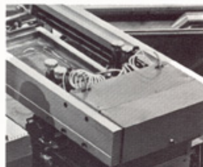
Squeegee/flood bar adjustments are made on the carriage.
