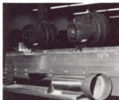
Magnum UV curing modules located between color stations.
