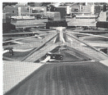
A rotary indexer automatically delivers substrates to each station.
