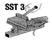
**SST 3 profiles** are designed with precision synthetic inserts and manufactured from wear-resistant materials to achieve optimal tension stability. Jaw pressure is controlled by a torque wrench allowing clamp strength to be easily adjusted for maximum mesh tension.
